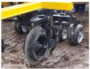
Figure 25: A Bio Blade or Cross slot<sup>™</sup> disc opener with opening disc and seeding tine, followed by paired press wheels. Note that the seed and fertiliser tube has sharp bends and may not be wide enough to avoid blockages when larger seeded pulses like faba or broad beans are being sown.
