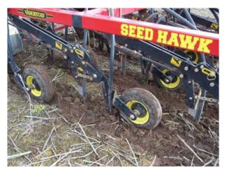
Figure 22: One of several seeding mechanisms for uniform sowing depth using the press wheel for depth control.
