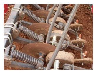
Figure 26: A Case IH SDX-40 single-disc drill.
