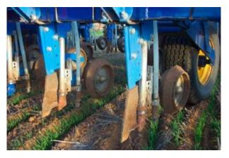
Figure 23: A Primary Precision Seeder fitted with hydraulic breakout for consistent penetration. It is also fitted with narrow points that form an 'inverted T' slot and is capable of deep or side placement of fertiliser.
