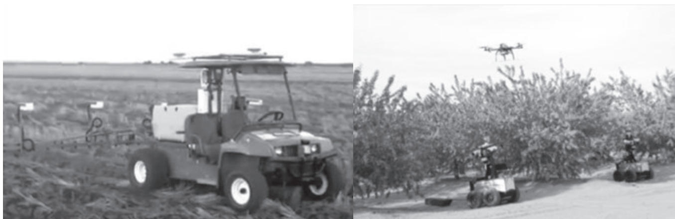
Figure 1. Small autonomous robot for zero-tillage agriculture (left), two ground robots and one aerial robot for crop surveillance in tree-crop applications (right).
