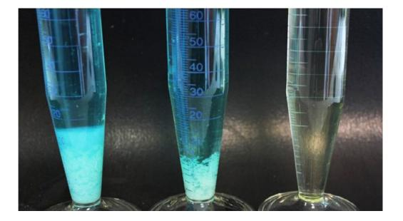
Three possible outcomes of the jar test: Left – layers forming, middle – sediment produced, right – well mixed
