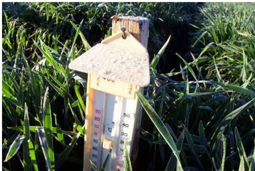
Photo 5: Canopy temperature measured using a calibrated minimum/maximum thermometer. For best results, a minimum of two or three field thermometers are required to give representative temperatures for a crop. In undulating country, more thermometers should be used to record temperatures at various heights in the landscape.
