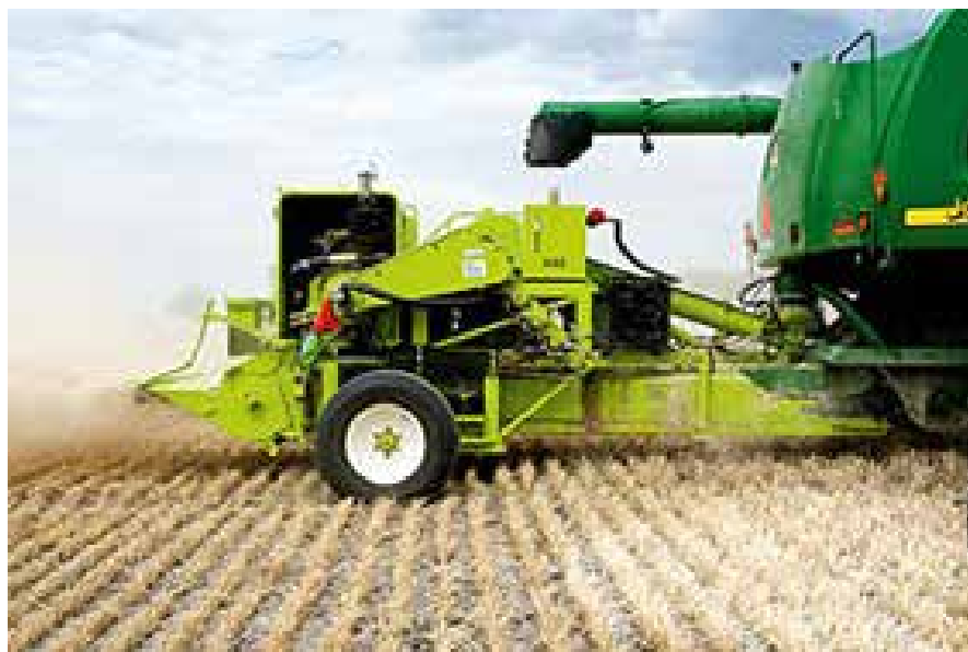
Photo 13: Harrington weed seed destructor at work in the paddock.
