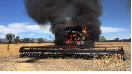
**Photo 16:** A harvester fire in a safflower crop. Like lentil and chickpea, harvesting safflower produces a fine dust meaning the risk of fire is great. (Photo: D. McLellan)
