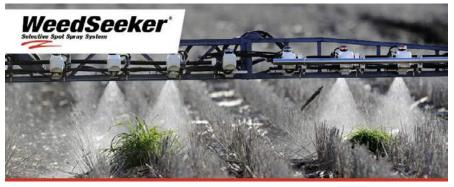
**Photo 21:** Selective sprayer technology, uses optical sensors to turn on spray nozzles only when green weeds are detected.
