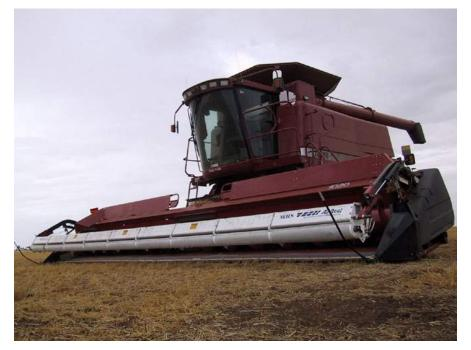
**Photo 2:** A harvester set up for lentil with a flexi-front and air assist. (Photo: W. Hawthorne, formerly Pulse Australia)
