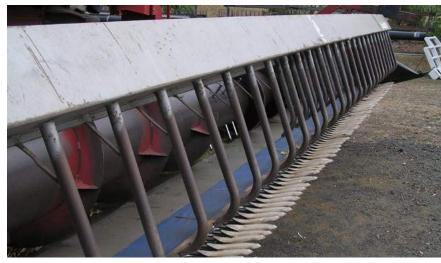
**Photo 4:** *Harvestaire front combined with extension fingers and a blue Vibra-mat.* (Photo: G. Cumming, formerly Pulse Australia)
