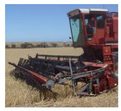
Photo 13: Rotary brush fitted to harvester to reduce snail contamination. (Photo: M. Richards)
