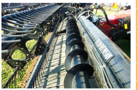
Photo 7: Belt front fitted with cross auger. Photo: W. Hawthorne, formerly Pulse Australia
