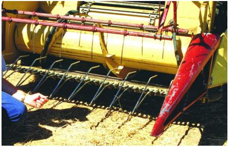
**Photo 5:** *Light crop lifters that can be used in lentils.* (Photo: G. Riethmuller)
