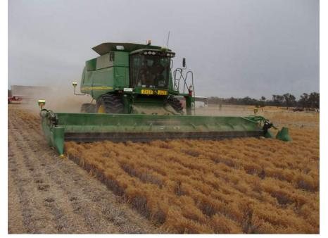
Photo 3: Harvesting lentil with a flexi-front and air assist. (Photo: T. Bray formerly Pulse Australia)
