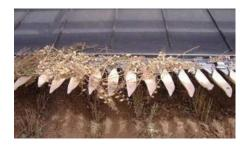
Photo 6: Plastic extension fingers fitted to a draper front. (Photo: G. Cumming, formerly Pulse Australia)
