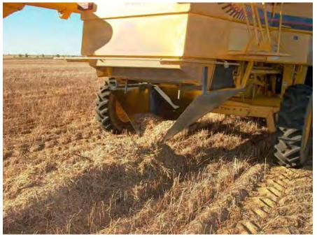
**Photo 2:** Directing chaff into a narrow windrow using a custom-made chute. Source: <u>GRDC</u>
