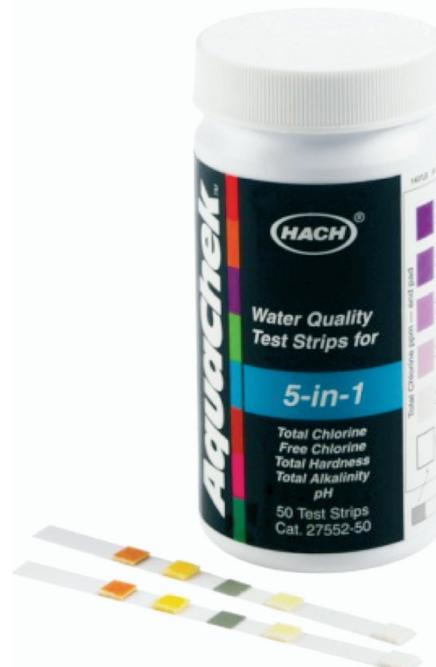
Water quality test strips can be used to assess pH and water hardness in the field.
