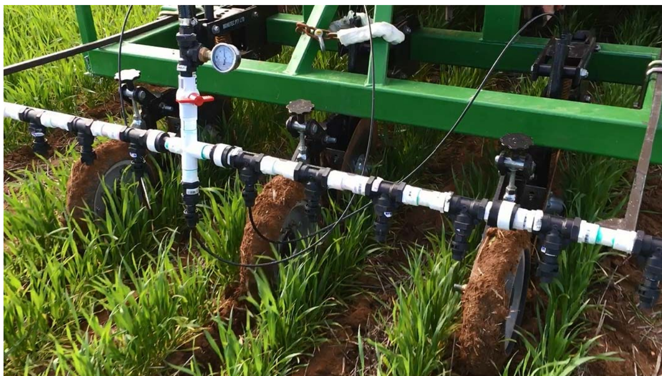
Figure 1. Fertiliser banding bar showing twin disc openers and press wheels with fertiliser spray boom (streaming and flat fan nozzle capable) at the rear.
