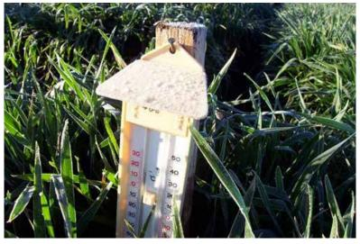
**Photo 3:** Canopy temperature measured using a calibrated minimum/ maximum thermometer. For best results, a minimum of two or three field thermometers are required to give representative temperatures for a crop. In undulating country, more thermometers should be used to record temperatures at various heights in the landscape.
