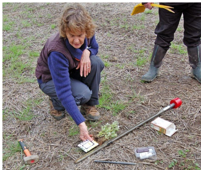
FIGURE 2.16 The ‘dig stick’ and a field pH test kit give a quick and convenient measure of soil acidity. Photo: M McClure
