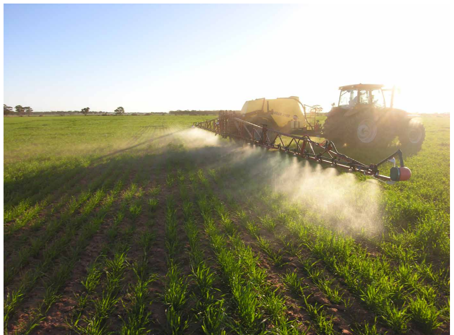
Photo 9: Using a boom spray on the crop when there is only a very light breeze helps prevent spray drift.
