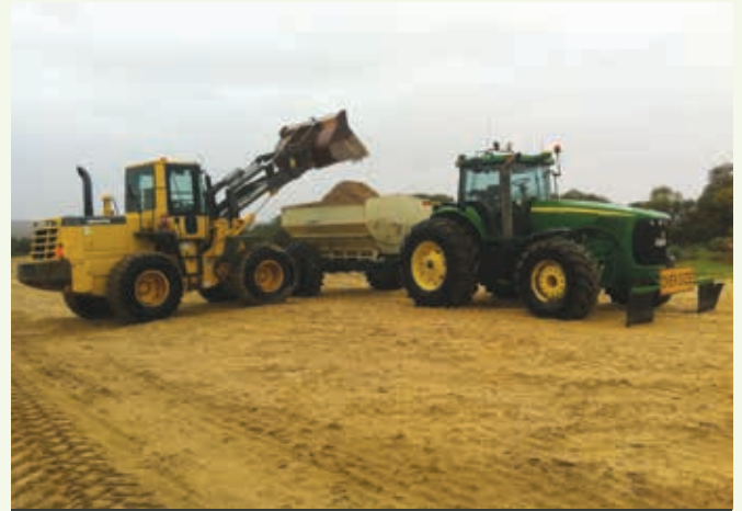
One of the Messina's two spreaders which are soon to be replaced with a single, 20–25t capacity unit
