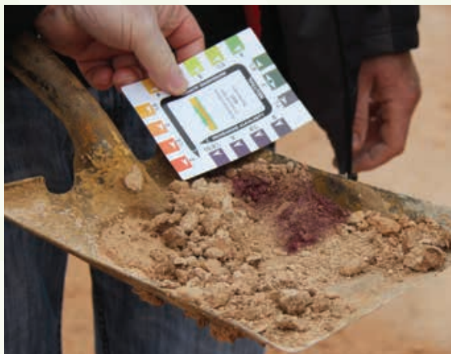
Using Universal indicator to measure the pH (in water) of the Morrel lime
