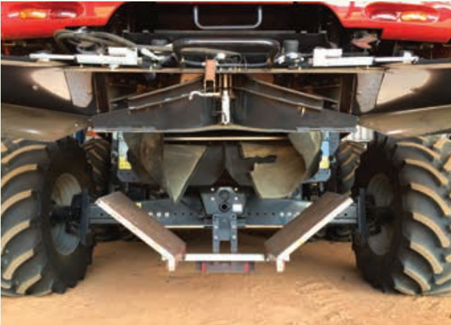
One of Rod's two Case 8240 headers set up with curtains and chute for windrowing harvest residue. (Photo courtesy of Ben White)
