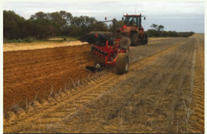
The Messina's 14-board, 6.2m wide Grégoire Besson mouldboard plough in action
