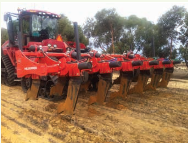
The Messina's 6m wide Grégoire Besson Heliripper capable of ripping to 800mm
