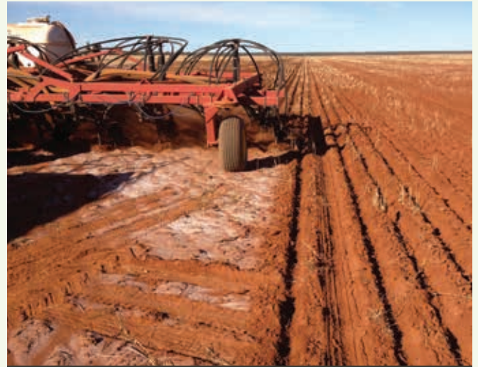
Seed Hawk® seeder in action after 2t/ha of applied lime during 2013. (Photo courtesy of Bill Crabtree)
