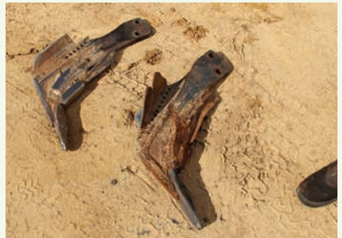
Peter’s ‘topsoil slotting’ system: ripper tynes with 75 x 75mm angle iron (left) or old scarifier points (right) welded behind the tyne
