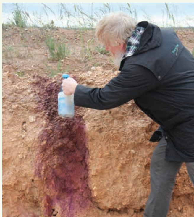
Chris Gazey (DAFWA) spraying the Morrel lime with Universal indicator. The dark purple colour indicates a pH of approximately 8 (in water) throughout the profile (NB: the shallow topsoil had been scalped from this area)
