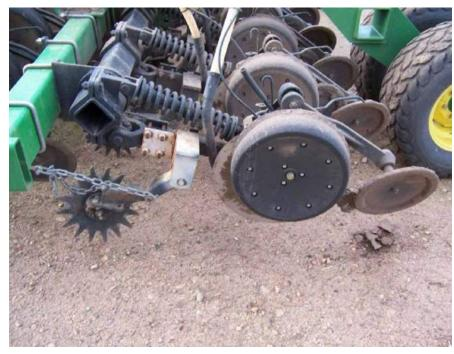
**Figure 10:** A disc seeder set up with Yetter trash clearing wheels and tubing for liquid injection of inoculum or trace elements during sowing. Note also the closer, to cover the seeding slot and act like a press-wheel from the side.
