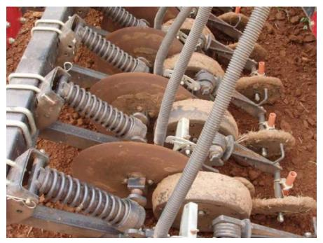
Figure 33: A Case IH SDX-40 single-disc drill.
