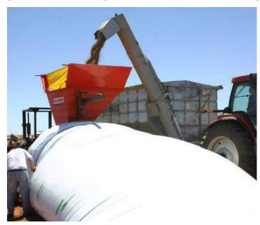
**Figure 6:** Silo bags (or grain, harvest bags) should be considered as only temporary storage for pulse grains because of quality issues that can arise.
