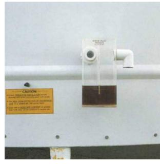
**Figure 5:** A gas lock on sealed silos gives a quick and reliable means of checking the seal of the silo. Some silos marketed as 'sealed' may not prove to be when tested.
