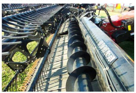
**Figure 2:** Belt-front fitted with cross-auger.
