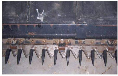
**Figure 3:** Short fingers on a flex-front.
