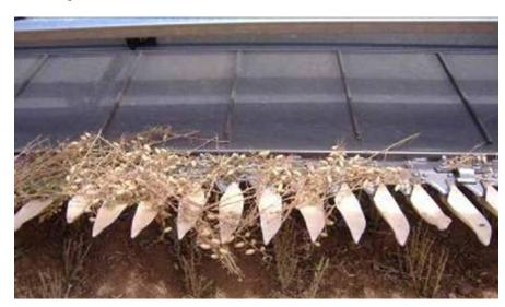
**Figure 4:** Plastic extension fingers fitted to a draper front.
