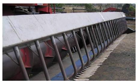
**Figure 5:** Harvestaire front combined with extension fingers and a blue vibra-mat. Photo: G. Cumming, Pulse Australia
