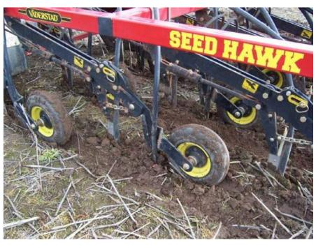
**Figure 32:** One of several seeding mechanisms for uniform sowing depth using the press-wheel for depth control.
