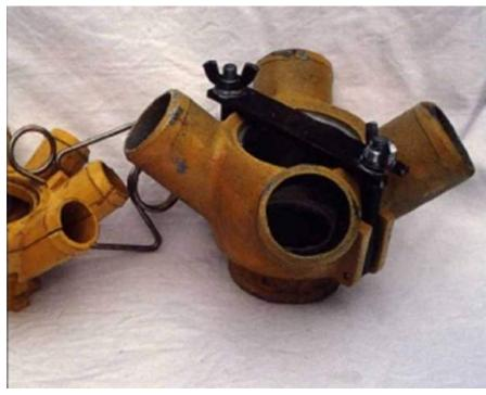
**Figure 31:** Conversion heads, such as this one for a Connor–Shea air seeder, allow large seeds such as faba beans and Kabuli chickpeas to be sown with ease.
