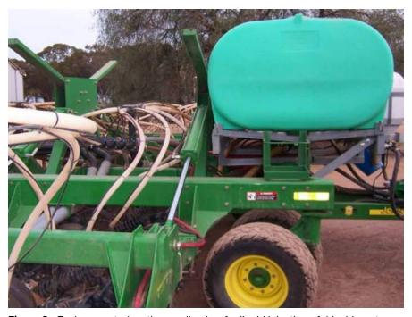
**Figure 9:** Tanks mounted on the seeding bar for liquid injection of rhizobia or trace elements during seeding. Agitation is required. Note the tubes and manifold. Inoculum must be applied under low pressure only. Some machines have their tanks set up as a separate, trailed tanker.
