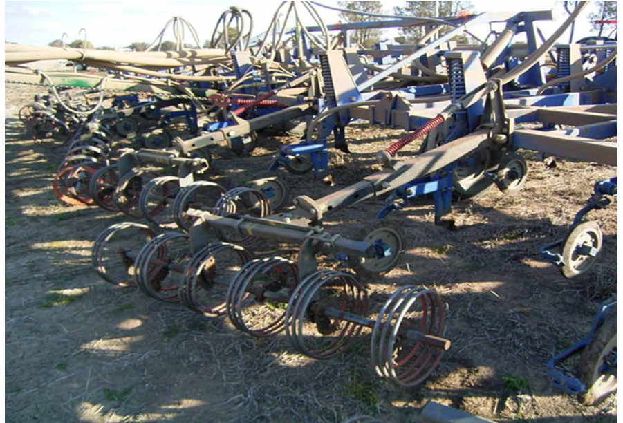
Figure 11: Rolling harrows on a zero-till rig setup for field pea sowing, Collie NSW.
