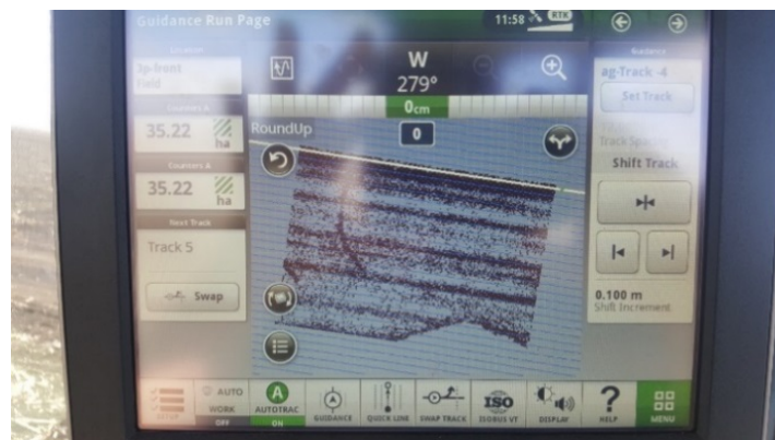
Figure 7. Spray map shown on spray controller
