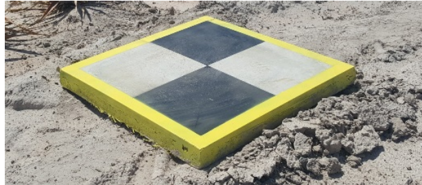
Figure 3. Ground control point
