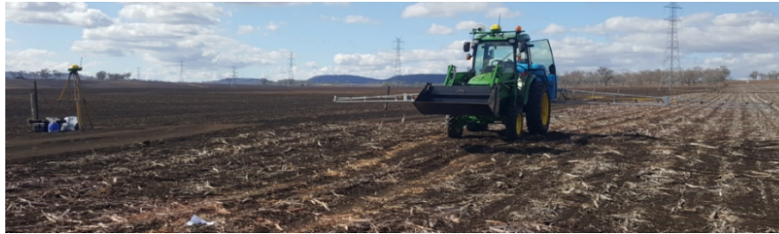
Figure 4. John Deere 4066R with link sprayer – base station is visible on the left
