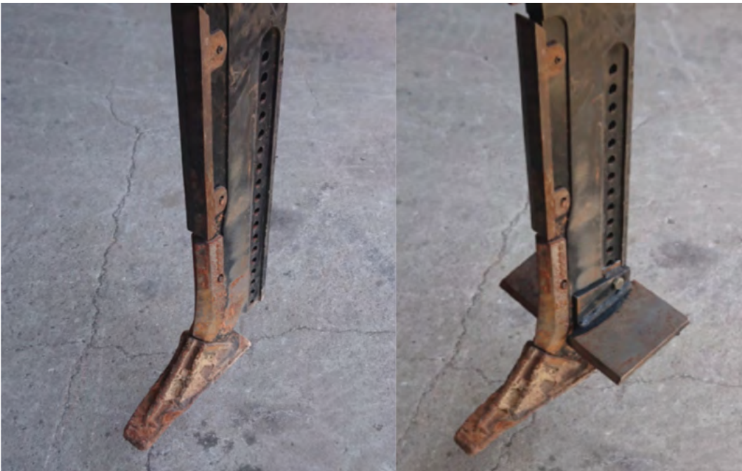
Figure 2. Ripper tine (left) and ripper tine with wings (right).
