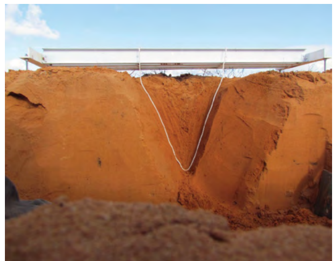
Figure 3. Excavated pit with a rope defining the boundary of the loosened soil area.
