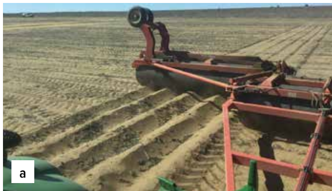
Figure 7: Rollers range from (a) flat steel rollers to (b) rollers mounted on deep ripping machines. Note the reduction in standing stubble following ripping and rolling in Figure 7b.
