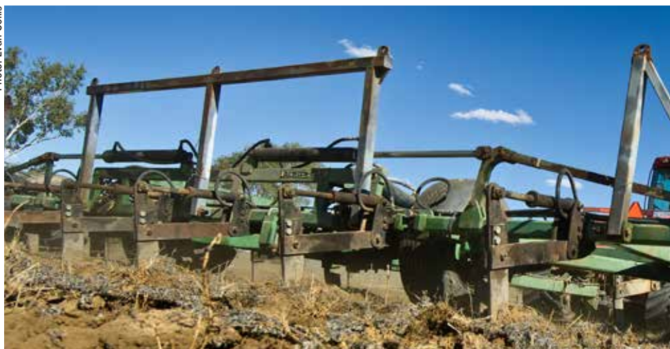
Some growers use deep ripping to ameliorate soil constraints that otherwise restrict the uptake of moisture.
