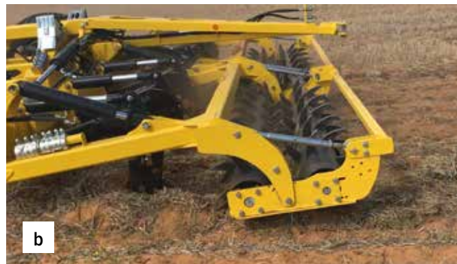
Figure 7: Rollers range from (a) flat steel rollers to (b) rollers mounted on deep ripping machines. Note the reduction in standing stubble following ripping and rolling in Figure 7b.
