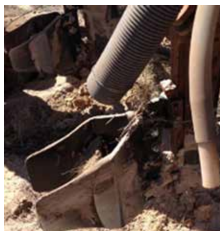
Figure 5: Topsoil inclusion plates fitted to deep ripping tynes on a Yeoman's Keyline Plough tynes.
