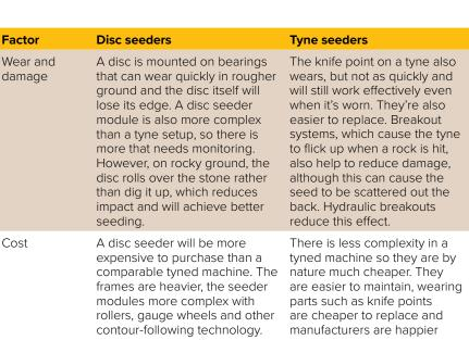
These costs are offset by the reduced amount of power (about 2hp per row less than a tyned seeder) needed to haul a disc seeder and the speed at which it can operate.
