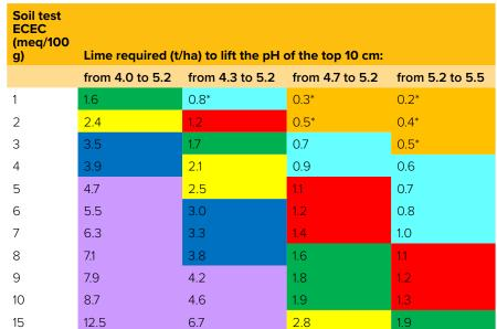
**Table 4:** Limestone required (fine and NV>95) to lift the pH of the top 10 cm of soilto 5.2. Colour codes group limestone rates to the nearest 0.5 t/ha.
