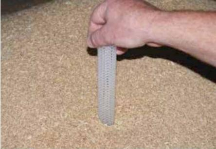
**Photo 8:** Probe traps pushed at the top of silos or bulk grain storages help detect the first signs of an insect infestation.
