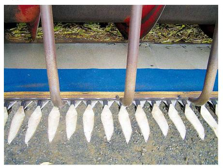
Photo 9: Plastic extension fingers fitted to harvester.
