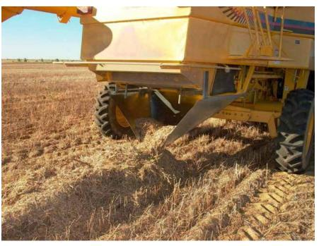
Photo 2: Directing chaff into a narrow windrow using a custom-made chute.
