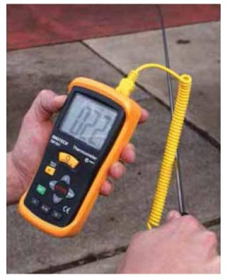
**Photo 6:** Monitor the effectiveness of the aeration cooling process by checking grain temperature with a temperature probe or a thermometer taped to a rod. Photo: Chris Warrick, Kondinin Group
