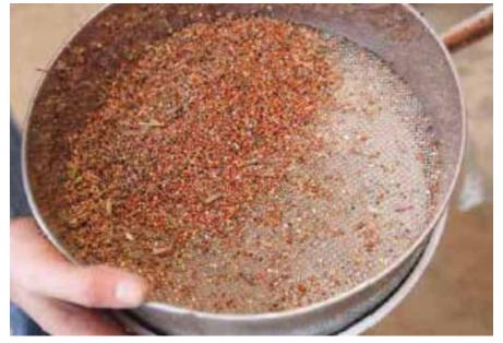
Photo 7: Use a 2 mm mesh sieve to separate insects from grain.
