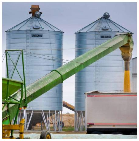
**Photo 1:** Storage sites, in particular silos, augers and trucks that have held treated fertiliser or alternate products such as pickled (treated) grain can be a source of potential contamination to otherwise clean grain subsequently loaded or moved through that equipment. Where possible, use different storages and augers to handle and store these products.
