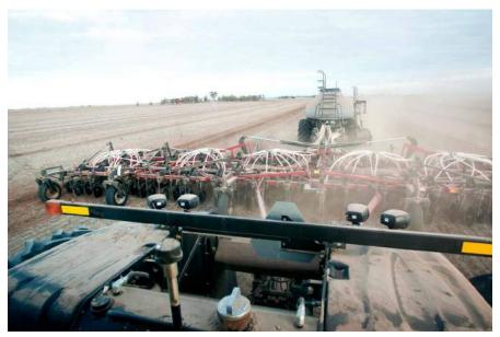
**Photo 7:** A New Holland T9 tractor with a Case Flexicoil PTX 600 airseeder bar towing a Flexi-Coil 3850 air cart bin used to sow seed.
