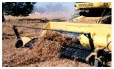
Photo 4: Harvesting narrow-leafed lupins using a pickup front. Source: <u>NSW DPI</u>
