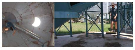
**Photo 4:** TIPS: An extended broom handle makes sweeping out silos easier (left). A concrete slab underneath silos makes cleaning easier. (right).
