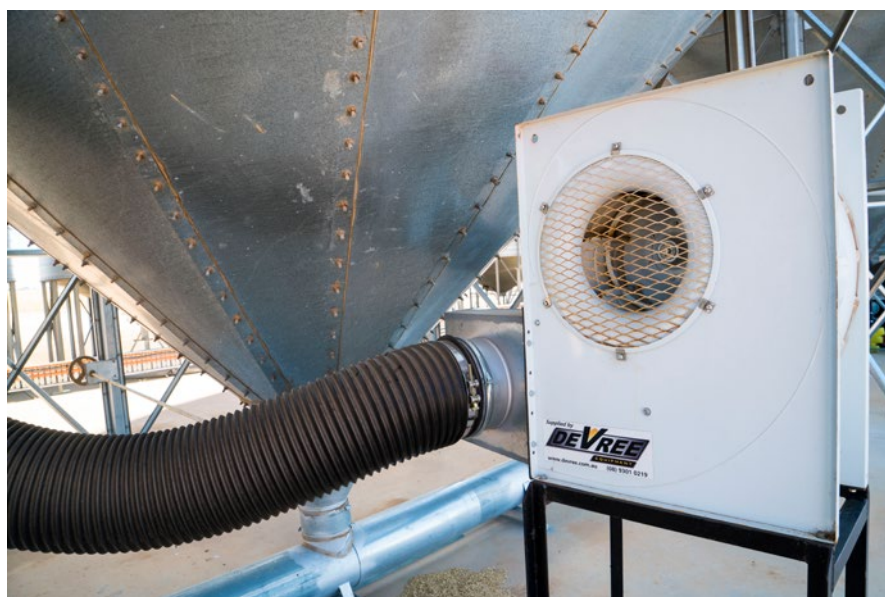
Photo 4: Silo fitted with aeration fan for cooling.
