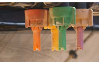
Single line multi-step system. The ARAG Selectron 4 nozzle system
