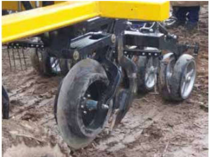
Photo 15: Bio Blade or Cross slot™ disc opener with opening disc and seeding tine, followed by paired press wheels. Note that the seed and fertiliser tube has sharp bends and may not be wide enough to avoid blockages when larger seeded pulses like faba or broad beans are being sown.
