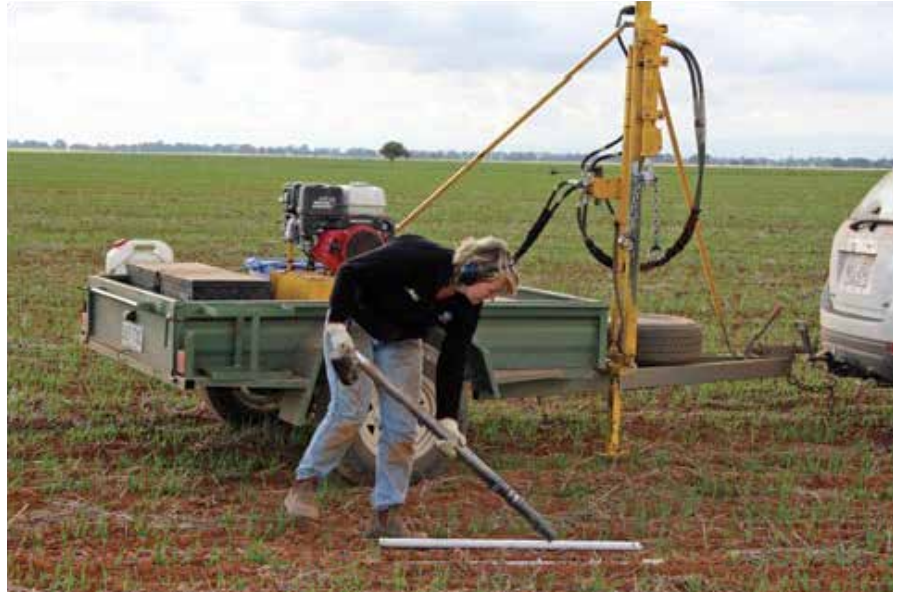
Photo 2: To be meaningful, soil sampling needs to take into account spatial variation in the soil condition. Differences in soil type, nutrient status and other soil properties may be exhibited within a paddock.
