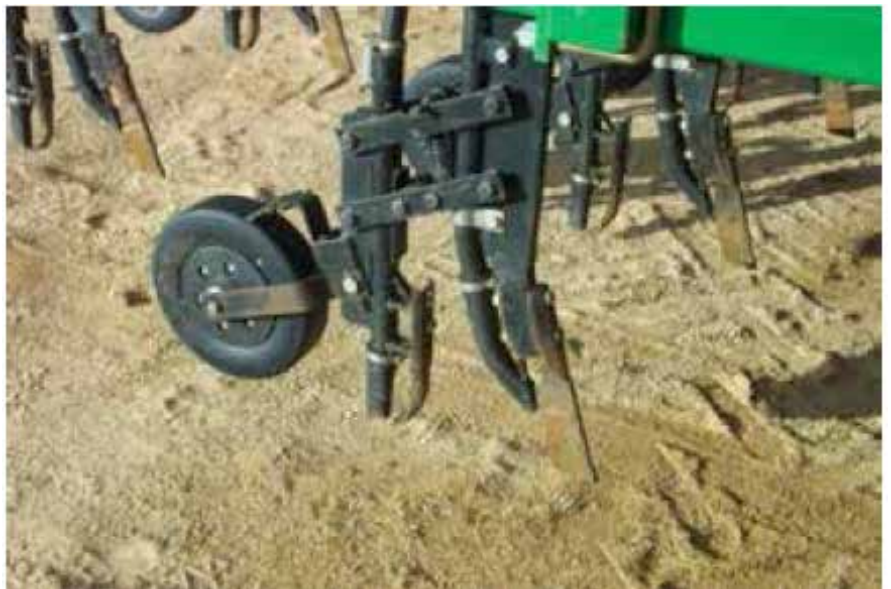
Photo 14: The DBS system parallelogram for uniform seeding depth and deep placement of seed or fertiliser.
