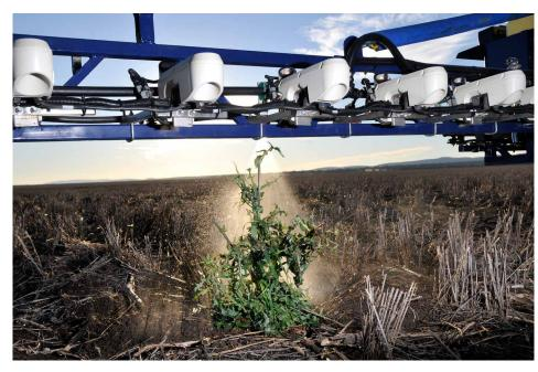
Figure 5: Selective sprayer technologies use optical sensors to turn on spray nozzles only when green weeds are detected. (Photo: CropOptics)
