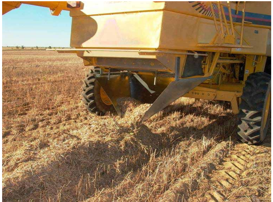
Photo 2: Directing chaff into a narrow windrow using a custom-made chute.
