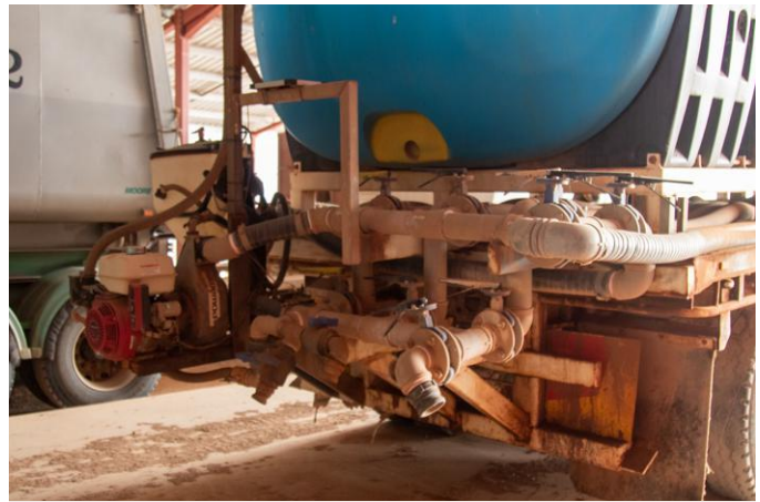
The plumbing system on the semitrailer, which contains three 15,000L tanks, allows for product mixing in the tanks (that is, the addition of trace elements) and it can fill the nurse trucks from either side. Photo: Petrina Ronald
