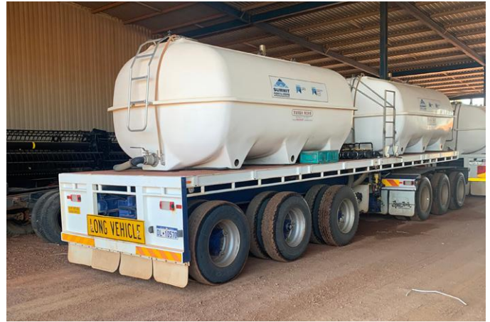
The Hathways' 12,500L UAN nurse tanks mounted on a 9m flat top trailer.
