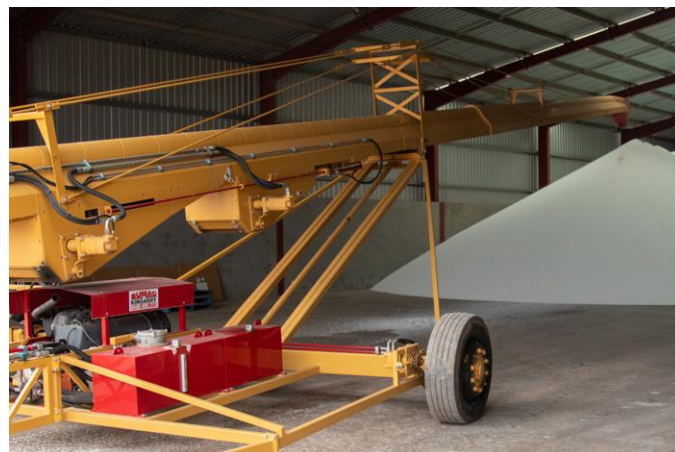
The 36m Sumac 38cm belt auger can unload 6t/minute.
