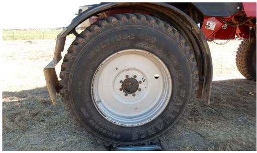
Before any increase to the tank size or boom width, consider the impact on the weight of the sprayer and the tyres required.
