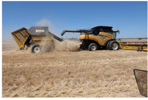
*Figure 7: Chaff cart in action, WA. (Photo: Trent Butcher, ConsultAg)* Chaff carts are towed behind headers during harvest to collect the chaff fraction as it exits the harvester (Figure 7). Collected piles of chaff are then burnt the following autumn or used as a source of stock feed. <sup>8</sup>
