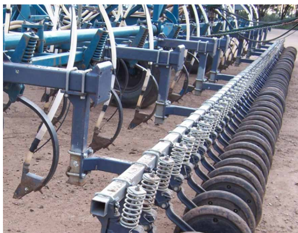
Figure 11: A seeder set up with Atom Jet narrow points, gang press wheels and liquid injection for either inoculum or trace element application during sowing.
