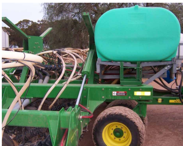
Figure 13: Tanks mounted on the seeding bar for liquid injection of either rhizobium or trace elements during seeding. Agitation is required. Note the tubes and manifold. Inoculum must be applied under low pressure only. Some machines have their tanks set up as a separate trailed tanker.
