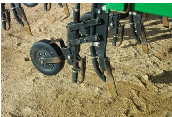
Figure 24: The DBS system parallelogram for uniform seeding depth and deep placement of seed or fertiliser.
