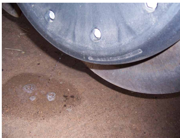
Figure 14: In furrow-liquid injection: Note the droplets from liquid injection, which can be used for either inoculating pulses or applying liquid trace elements. (Source: Grain Legume Handbook)
