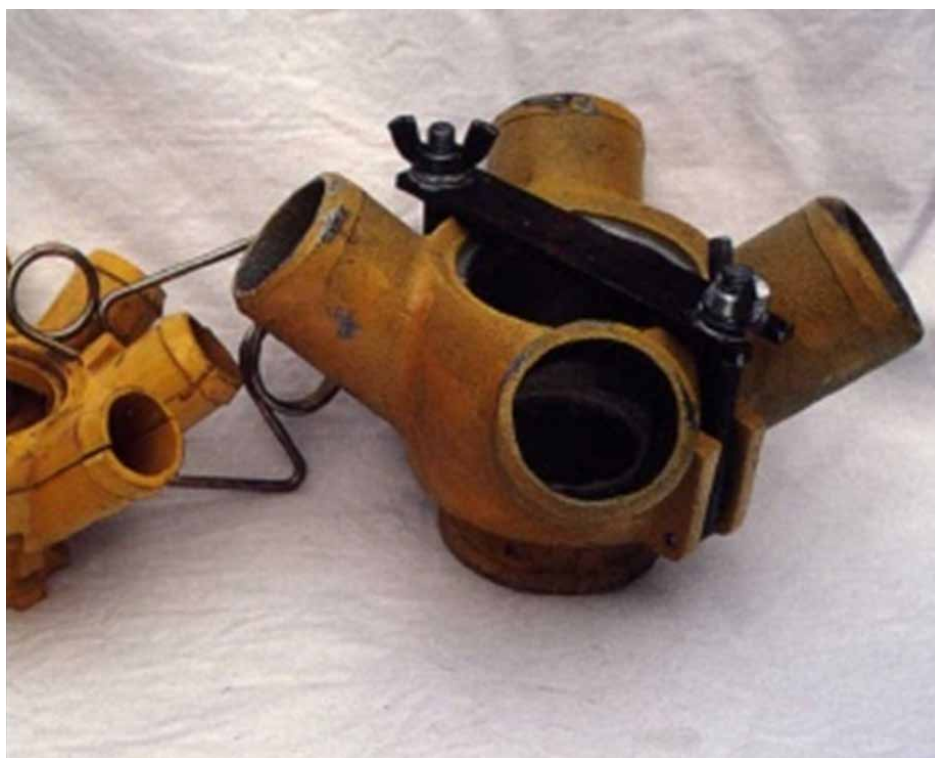
Figure 21: Conversion heads, such as this one for a Connor-Shea airseeder, allow large seeds such as broad beans, faba beans and Kabuli chickpeas to be sown with ease. (Source: Grain Legume Handbook, http://www.grdc.com.au/uploads/documents/3 Seeding.pdf )
