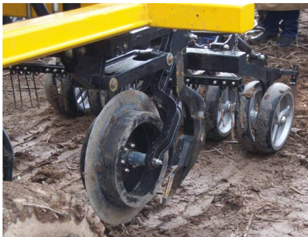
Figure 25: A Bio Blade or Cross slot™ disc opener with opening disc and seeding tine, followed by paired press wheels. Note that the seed and fertiliser tube has sharp bends and may not be wide enough to avoid blockages when larger seeded pulses like faba or broad beans are being sown.
