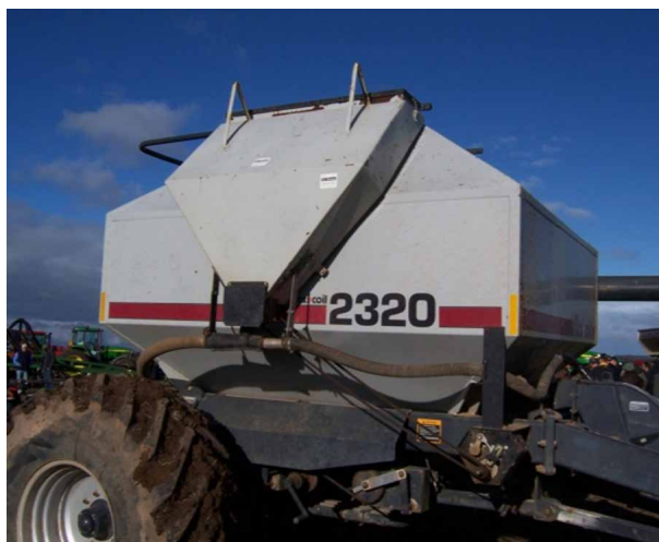
Figure 15: An 'after-market' third box fitted to a Flexicoil box to enable application of granular inoculums. Note that granular inoculums cannot be applied mixed with the seed (uneven distribution of seed and/or inoculums occurs). Rhizobial survival is severely jeopardised if granular inoculums are applied mixed with fertiliser. (Source: Grain Legume Handbook)
