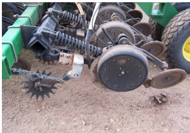
Figure 12: A disc seeder set up with Yetter trash clearing wheels and tubing for liquid injection of either inoculum or trace elements during sowing. Note also the closer to cover the seeding slot and act like a 'press' wheel from the side.
