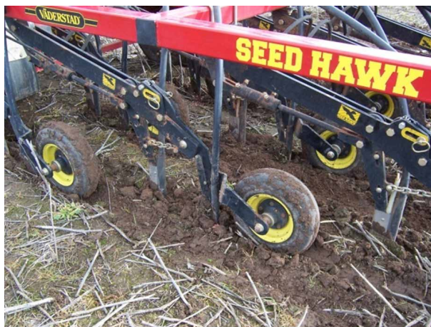
Figure 22: One of several seeding mechanisms for uniform sowing depth using the press wheel for depth control.
