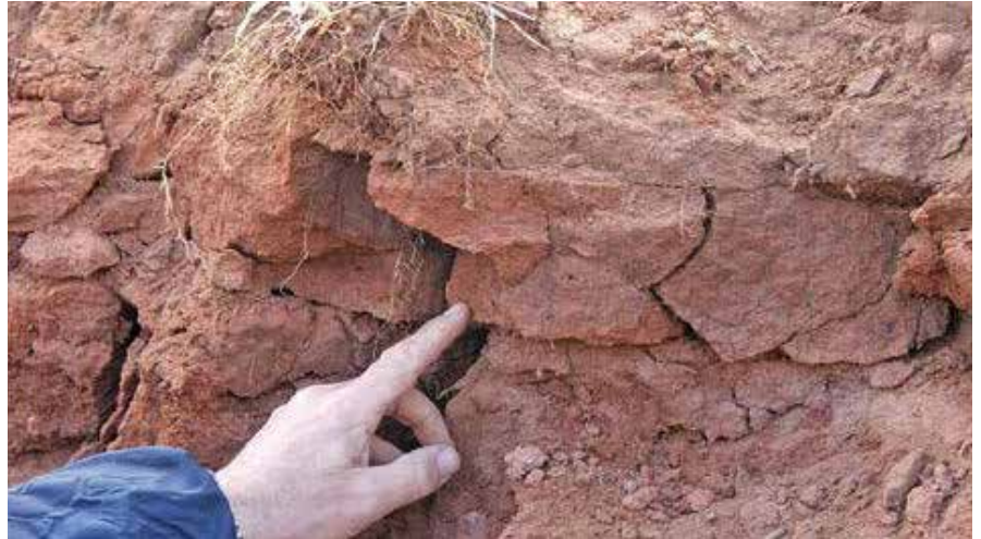
Photo 6: A distinct compacted layer in a sandy loam. Note fractures in hard pan through which roots prefer to grow.
