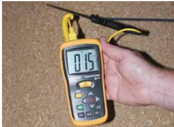
Photo 4: Monitor moisture and temperature using a digital probe from both the top and the bottom of silos, if safe to do so.
