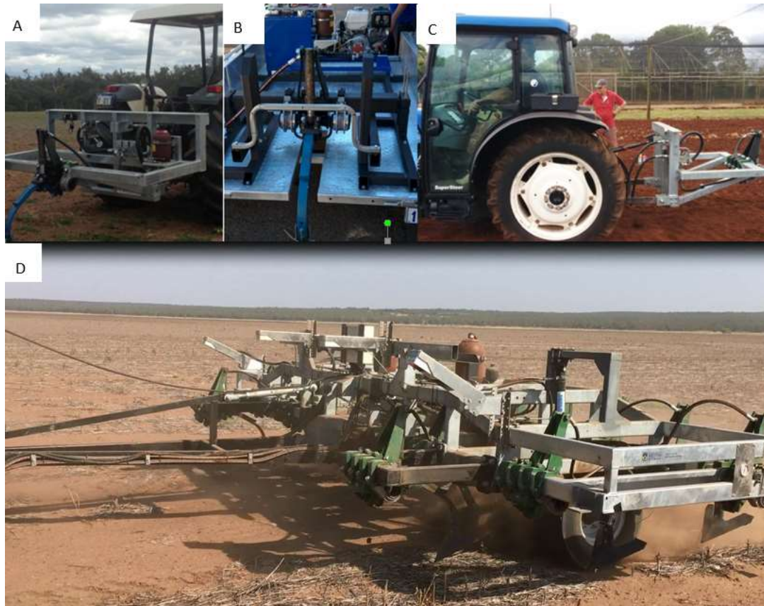
Figure 1. Initial proof-of-concept rig (Shenton Park) (A), Narrabri trailer mounted self-powered rig (B) and QDAF 3-point-linkage rig (C) and Pre-commercial rig – the ‘Weed Chipper’ (D) used in the testing and validation of targeted tillage fallow weed control.
