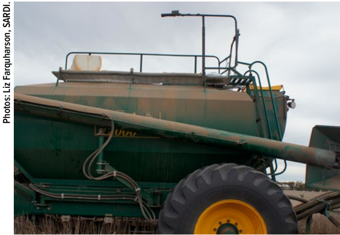
FIGURE 2-14 (a). A seeder allowing separation of seed, fertiliser and rhizobia granules prior to seeding.
