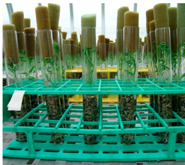
FIGURE 6-2. Plant assay method for counting rhizobia in soil. Plants are inoculated with different soil dilutions and the frequency of nodulation measured.
