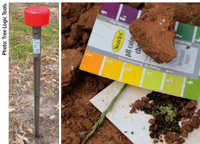
FIGURE 2-22 (left). A ‘dig-stick’ can be used to get a soil core to test pH and identify acidic soil conditions. FIGURE 2-23 (right). Garden centre pH kit.
