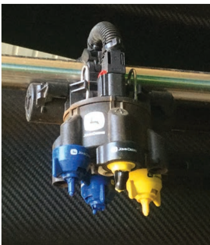
1. John Deere's ExactApply™ is a good example of the latest engineering and modularity with multiple spraying systems within one carousel unit. It contains a standard spraying system, multi-step system and PWM.
