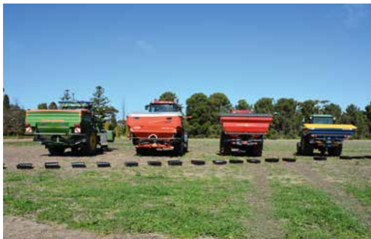
A snail bait distribution trial on Yorke Peninsula in 2013 tested the coverage of Amazone, Bogballe, Kuhn and Vicon urea spreaders with Meta, Metarex, Slugger and Slugout snail baits.
