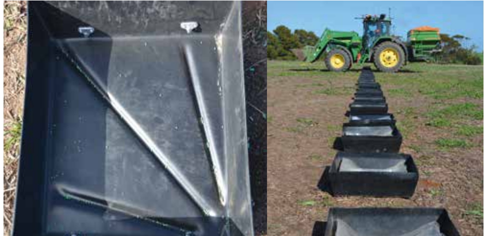
A series of black trays were set up to catch the snail bait as it was distributed by each spreader. The baits captured in each tray were collected and the weight measured and recorded to compare efficiency.
