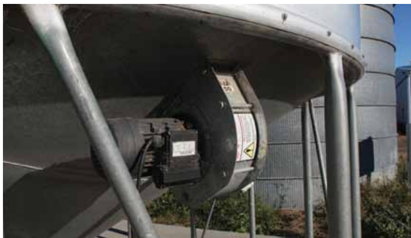
Air on: Aeration cooling is essential for storing oilseed and may require extra capacity to achieve 2–3 l/s/t in small oilseeds like canola.
