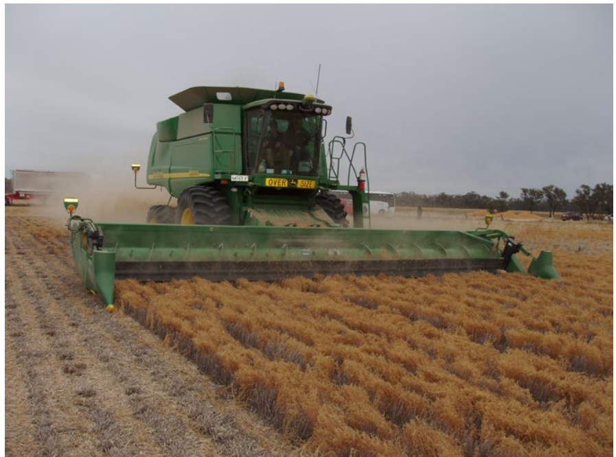
Photo 3: Harvesting lentil with a flexi-front and air assist.
