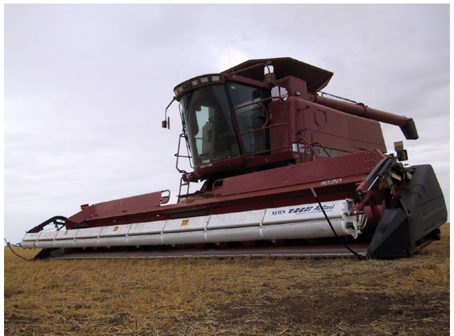
Photo 2: A harvester set up for lentil with a flexi-front and air assist.
