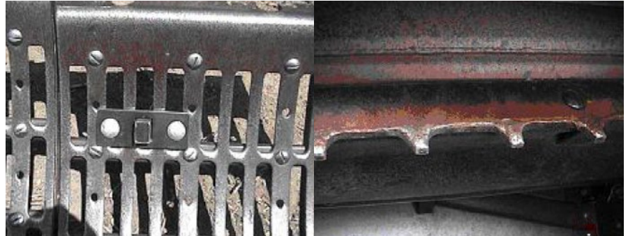
Photo 11: Disrupter peg (left) and disrupter bar (right) fitted to harvester for early bean harvest.
