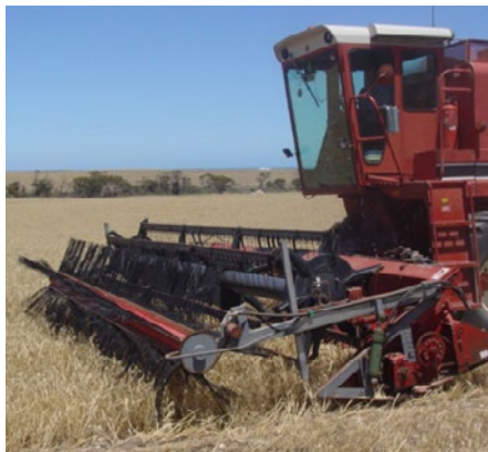
Photo 13: Rotary brush fitted to harvester to reduce snail contamination.
