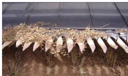
Photo 6: Plastic extension fingers fitted to a draper front.
