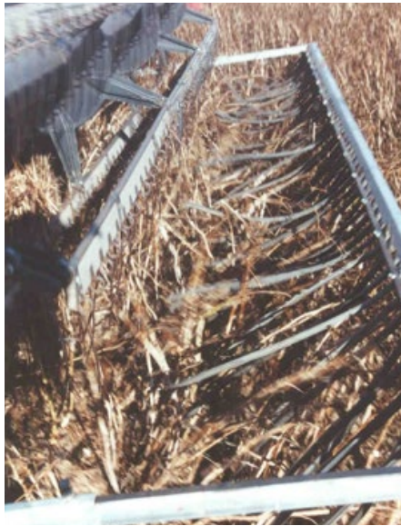
Photo 12: Pusher bar with dangling belts fitted to harvester to reduce snail contamination.
