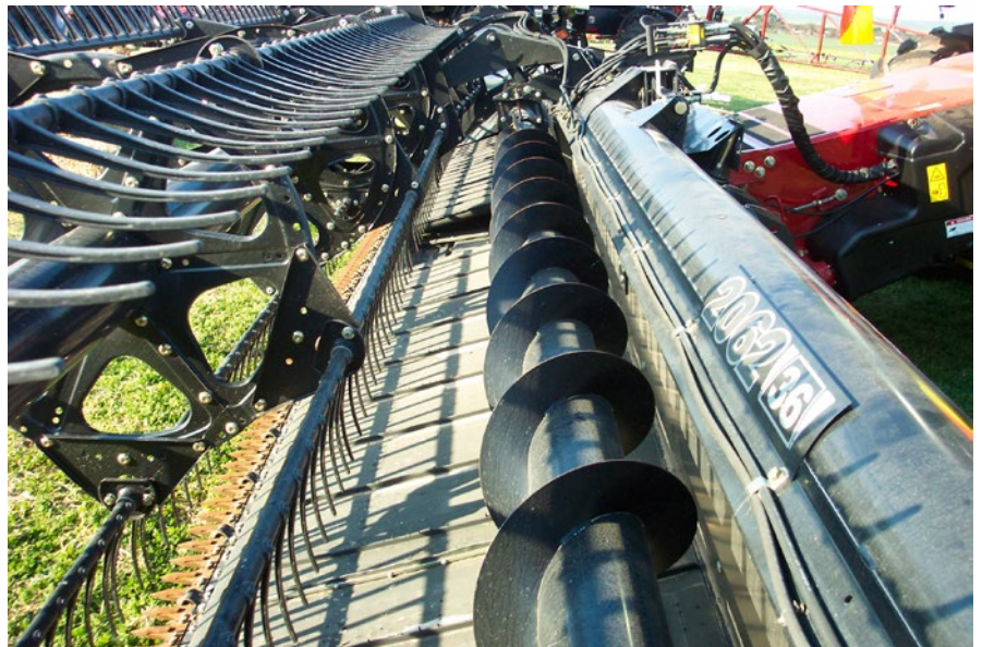
Photo 7: Belt front fitted with cross auger.
