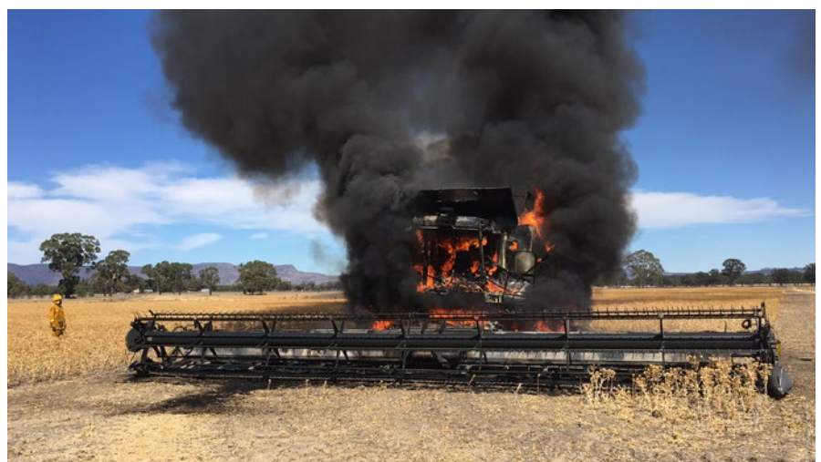
Photo 16: A harvester fire in a safflower crop. Like lentil and chickpea, harvesting safflower produces a fine dust meaning the risk of fire is great.
