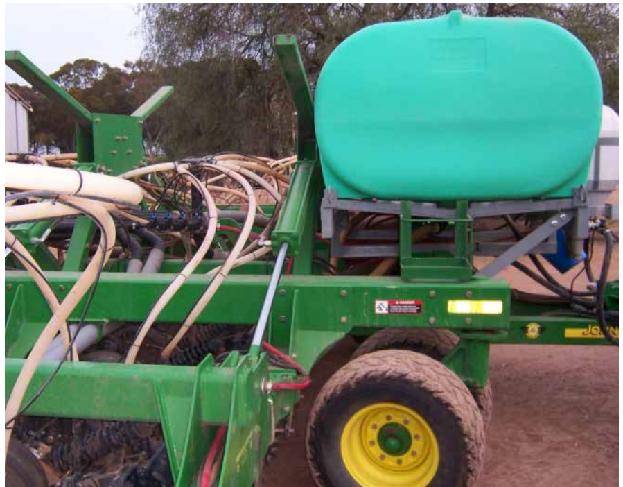
Photo 6: Tanks mounted on the seeding bar for liquid injection of rhizobia or trace elements during seeding. Agitation is required. Note the tubes and manifold. Inoculum must be applied under low pressure only. Some machines have their tanks set up as a separate, trailed tanker.
