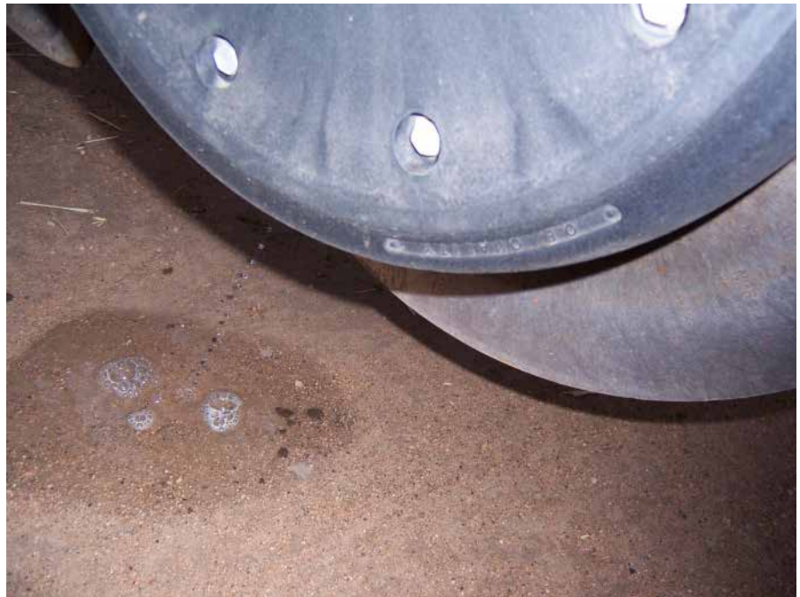
Photo 8: In-furrow liquid injection. Note the droplets from the liquid injection, which can be used for inoculating pulses or applying liquid trace elements.
