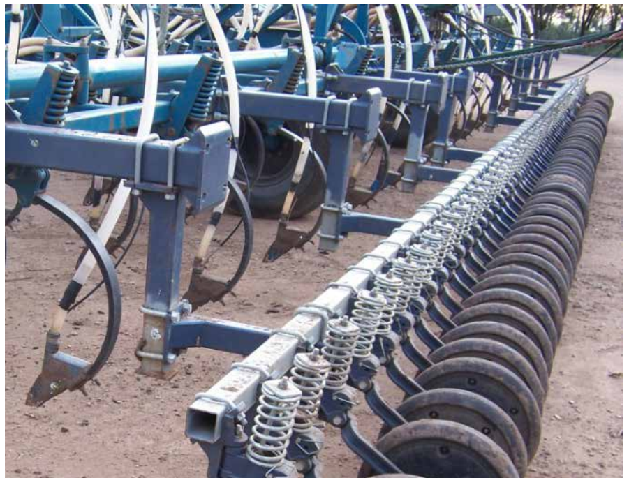
Photo 5: A seeding bar setup with Atom Jet narrow points, gang press-wheels and liquid injection for either inoculum or trace element application during sowing.
