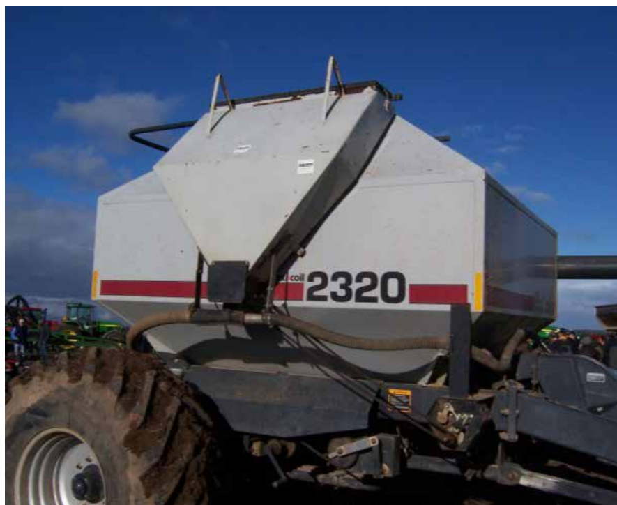
Photo 9: An 'after-market' third box fitted to a Flexicoil box to enable application of granular inoculum.
