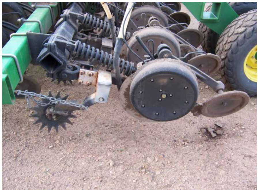
Photo 7: A disc seeder set up with Yetter trash-clearing wheels and tubing for liquid injection of inoculum or trace elements during sowing. Note also the closer, covering the seeding slot to act like a press-wheel from the side.
