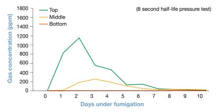
Figure 3: Gas concentration is poor over the 10 days in a non-gas-tight silo. (Source: QDAFF) To find out more about how to pressure-test silos, visit 'Fumigating with phosphine, other fumigants and controlled atmospheres' at <a href="DAFWA">DAFWA</a> (2015) Oats: harvesting, swathing and grain storage.
