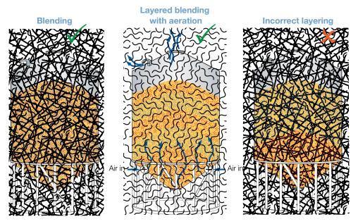
Figure 11: Correct blending. (Source: Kondinin Group)
