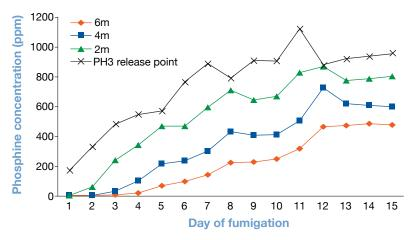
Figure 8: Spread of phosphine gas in a silo bag from a release point to gas monitoring lines at 2, 4 and 6 m along a silo bag.
