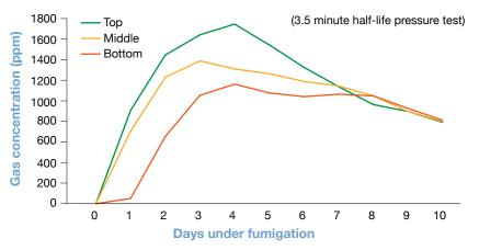
Figure 2: Good gas concentration maintained over time in gas-tight sealable silo. (Source: QDAFF)
