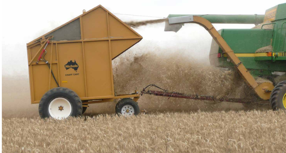
Figure 5: Chaff carts towed behind the header to catch weed seeds. (Photo: Cox Inall)
