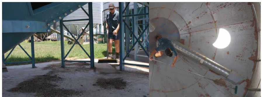
Photo 7: TIPS: An extended broom handle makes sweeping out silos easier (left). A concrete slab underneath silos makes cleaning easier. (right).
