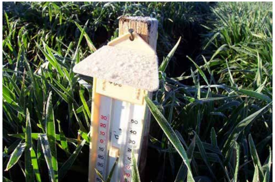
Photo 7: Canopy temperature being measured using a calibrated minimum-maximum thermometer. For best results, a minimum of two or three field thermometers are required to give representative temperatures for a crop. In undulating country, more thermometers should be used to record temperatures at various heights in the landscape.
