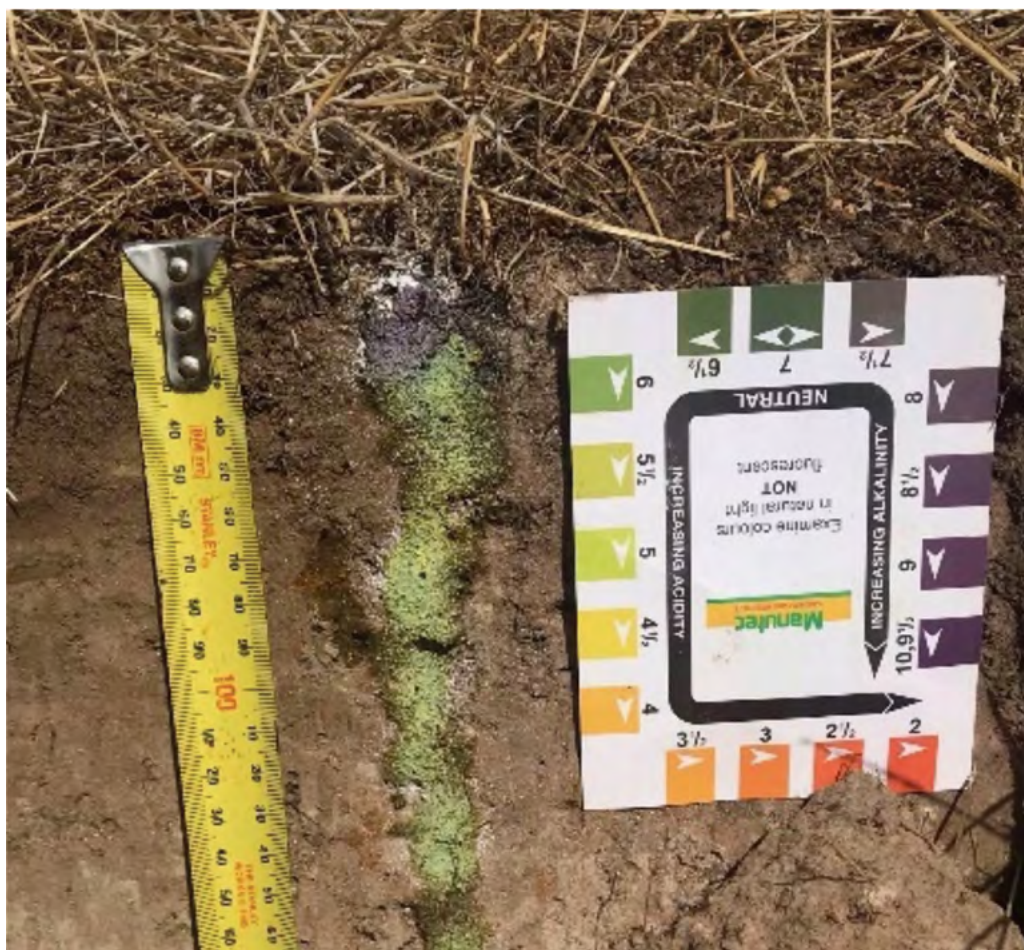
Figure 2. Example soil pit face with pH indicator dye applied. An alkaline surface layer can be seen (purple), overlying acidic soil (bright green) below 3cm.
