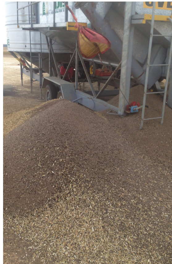
A pile of small conical snails removed from canola using a 4-barrel rotary grain cleaner with 2.5mm slotted screens.
