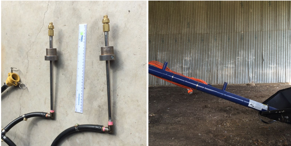
Figure 5. Spray application equipment designed for good coverage by applying treatment at two points in the auger
