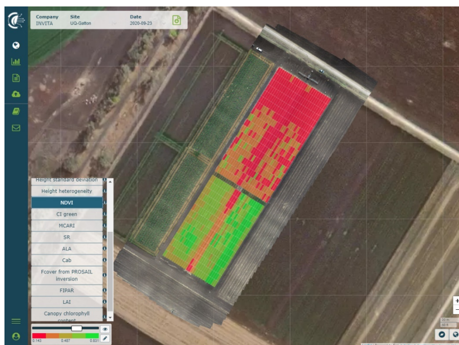
Figure 3. Example of NDVI per plot data collected from analysis of a single UAV drone flight at UQ Gatton. This image is stitching together multiple images taken by a drone in a ‘lawnmower’ pattern that takes about 30 minutes per ha at this high resolution.
