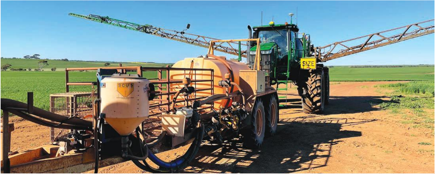
The repurposed Beverley Hydra Boom acts as a semi-concentrate hot mix tank which is pulled behind the water truck.
