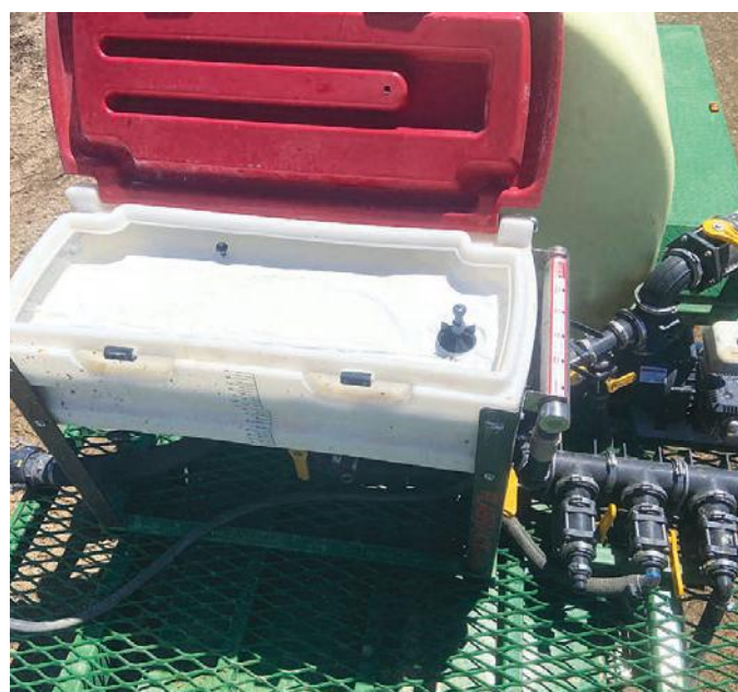
The Flash Vat 180L mixing vat features options for drum rinsing, vat rinsing and vat agitation, and a hand wash gun.
