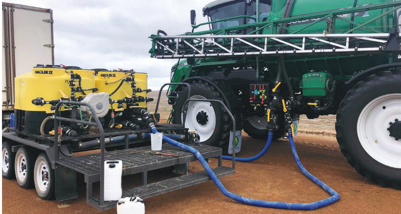
While the sprayer is being filled, the spray operator is batching the next load for the second sprayer.
