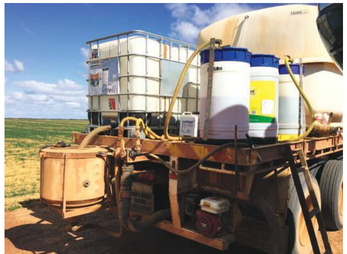
The nurse truck trailer is loaded up with a 1000L IBC shuttle and 110L Enviro Drums linked to the cone-bottom measuring vat, which inducts directly into the pump where the chemical is mixed with water and pumped to sprayer.
