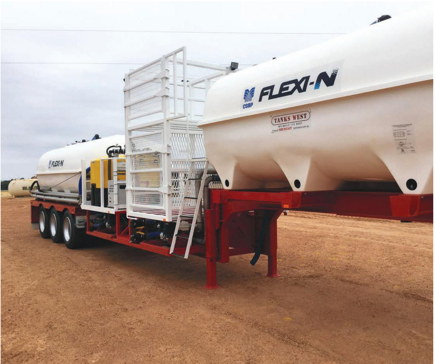
The drop deck trailer carries 27,000L of water and is equipped with a Handler IV 870L batching system.
