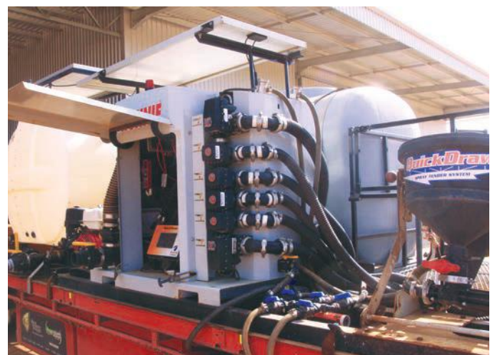
The SurePoint QuickDraw pre-programmed automated batching system replaces manual measurement of product amounts.
