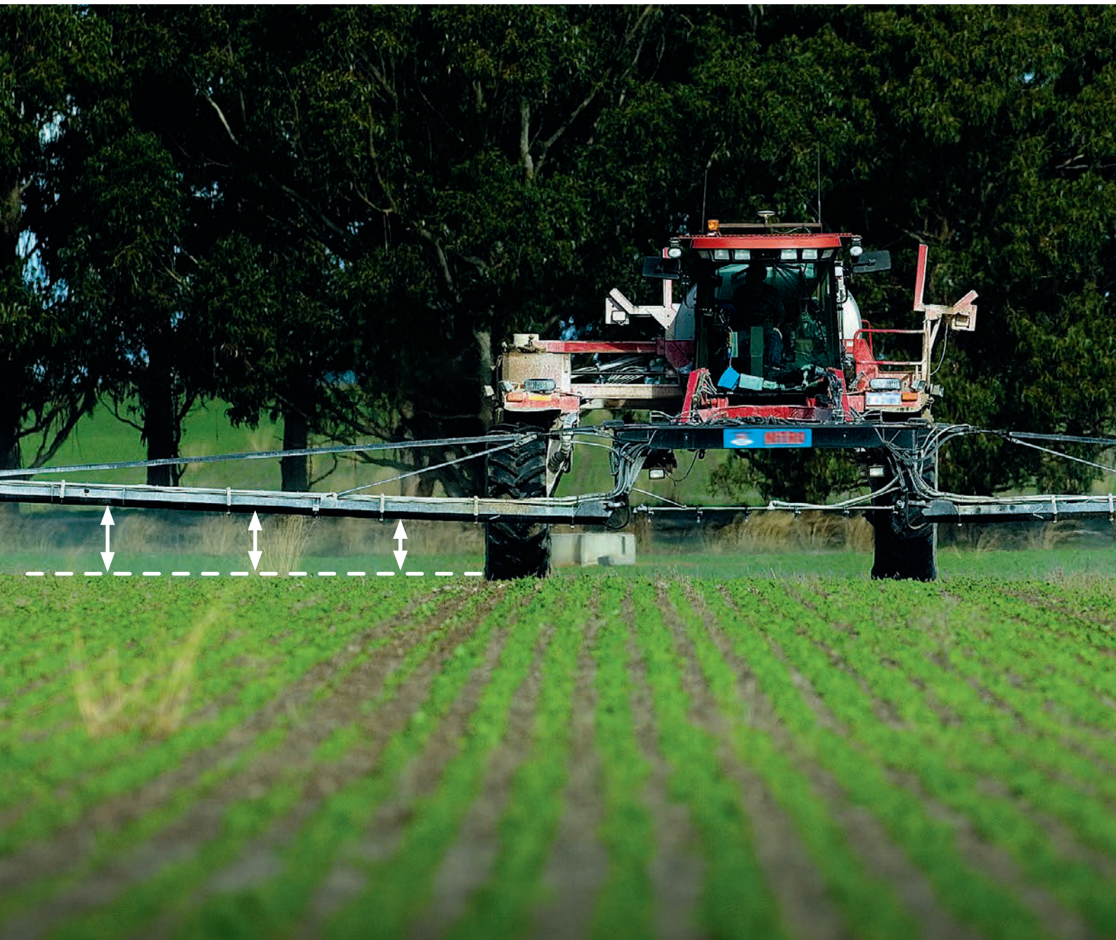
Increasing boom height increases drift risk.
