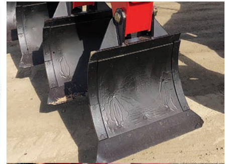
Figures 3a (top) and 3b (bottom): TATU reversible square plough.
