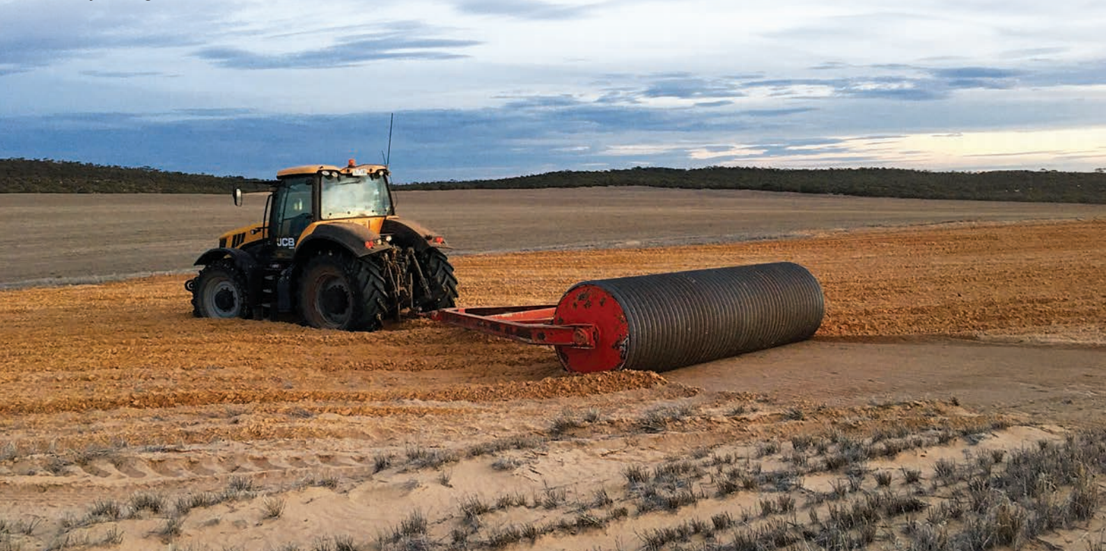
Figure 10: Post-ploughing rolling operations at Cowangie, Victoria, challenged by sinkage and traction limitations due to soft seedbed
