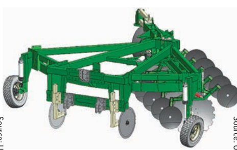
Figure 2a: John Shearer prototype two-way high work rate disc plough with concave disc skimmers.
