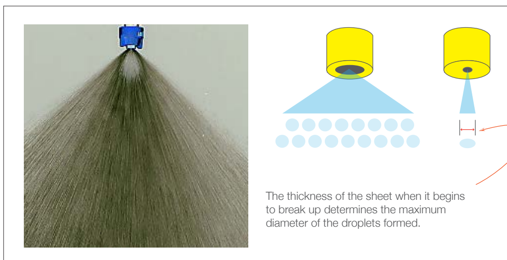
Figure 8 Sheet break-up into droplets from a flat-fan nozzle.
