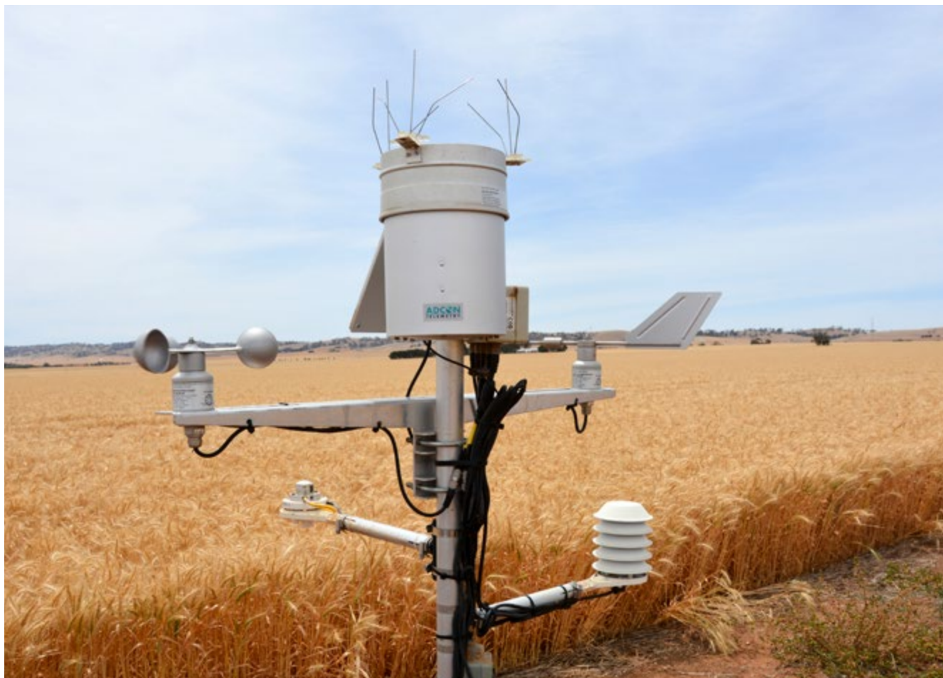
Soil moisture probes and weather stations can provide useful in-season data for decision-making. PHOTO: GRDC
