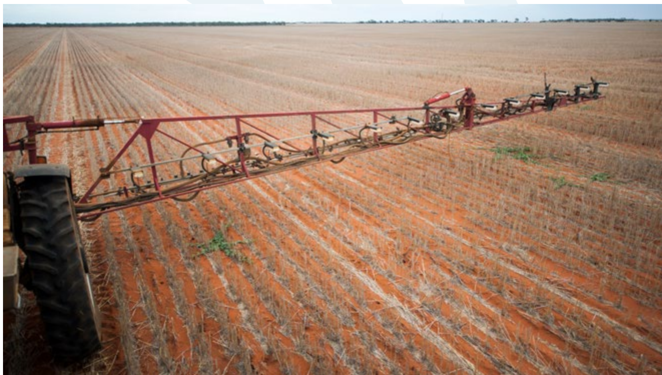
Technologies such as precision herbicide application using a WEEDit machine are making summer weed control more efficient and affordable in the eastern grainbelt. PHOTO: GRDC
