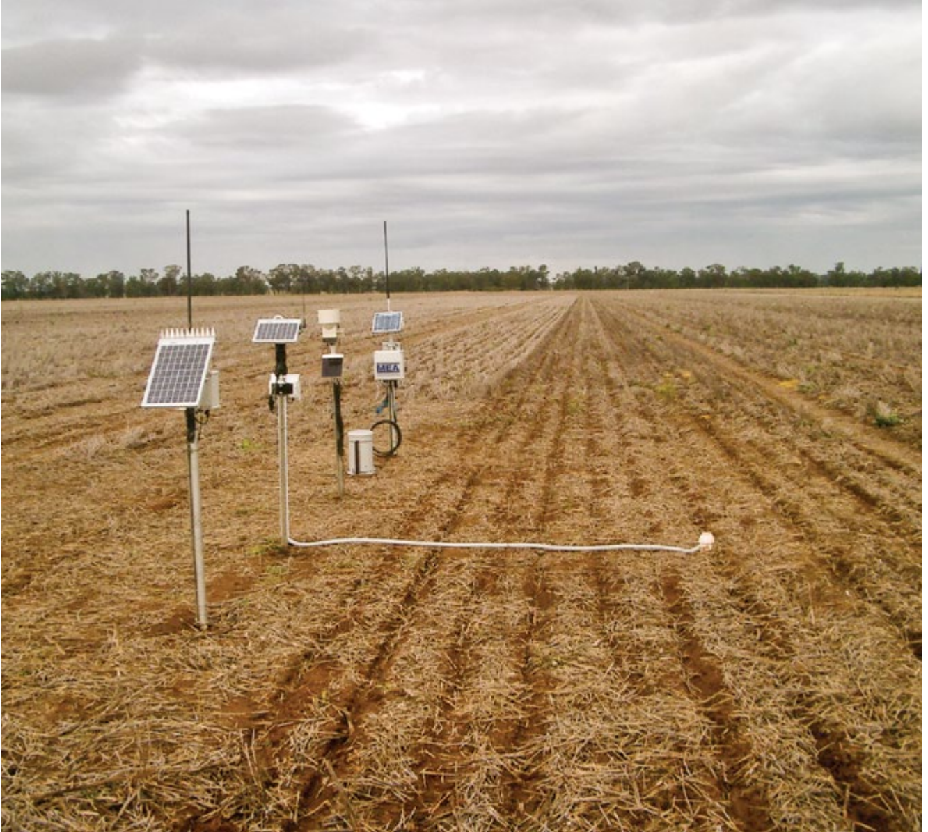
Soil moisture probe systems, similar to these, are set up on the Aynsley's property to help characterise soil types. PHOTO: GRDC
