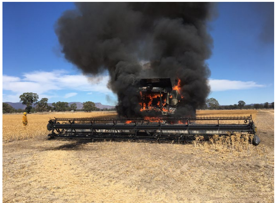
Photo 16: A harvester fire in a safflower crop. Like lentil and chickpea, harvesting safflower produces a fine dust, meaning the risk of fire is great.
