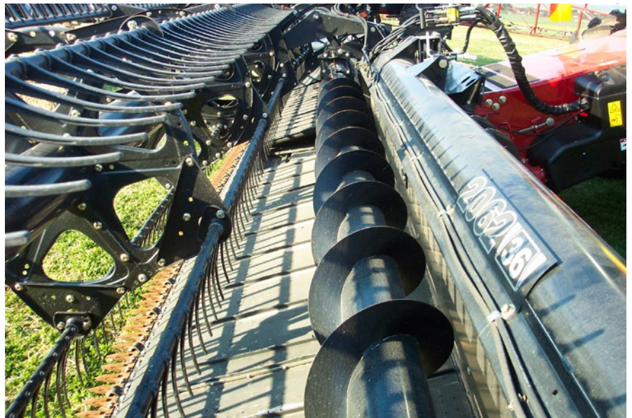
Photo 7: Belt front fitted with cross auger.
