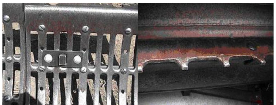
Photo 11: Disrupter peg (left) and disrupter bar (right) fitted to harvester for early bean harvest.
