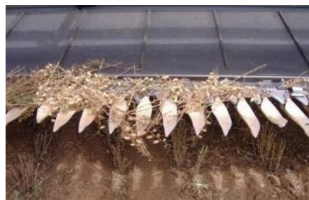
Photo 6: Plastic extension fingers fitted to a draper front.
